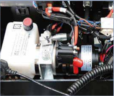
Integrated hydraulic unit, compact structure, less space
